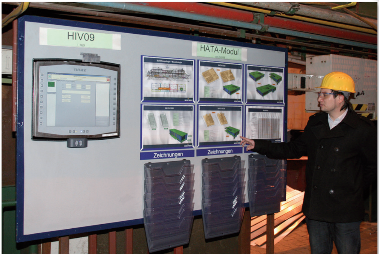
Interface between planners, logistics specialists and mechanics – here in the shipbuilding industry: Visualisation Board with integrated touch screen
